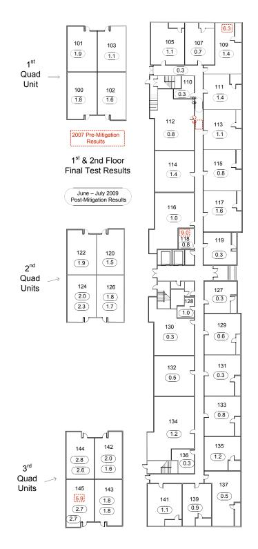
Figure 8 First Floor Final Radon Measurements
