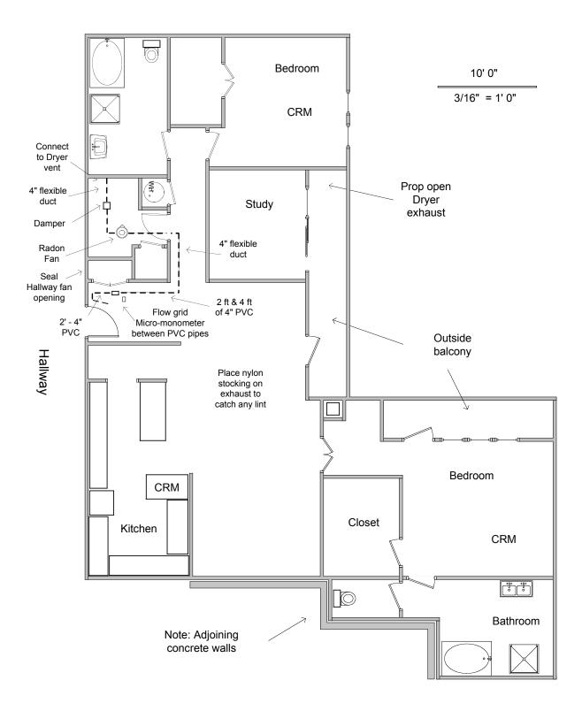
Figure 1 Unit 504 Floor Plan & Ventilation Test
