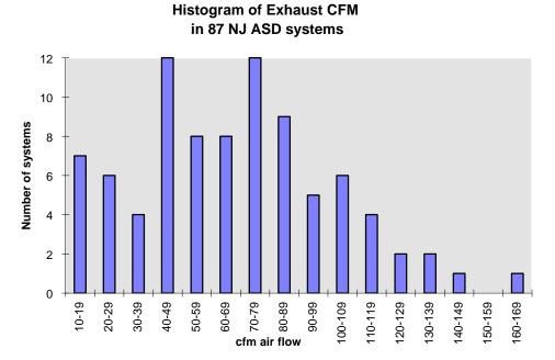
Figure 1 - ASD system Airflow from NJ study of mitigated houses
