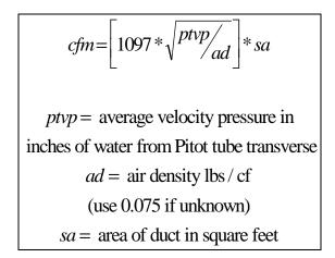
Formula 1 - CFM determination from transverse Pitot tube reading
