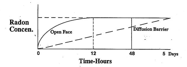
Figure 1. How Charcoal Works as an Equilibrium Material
