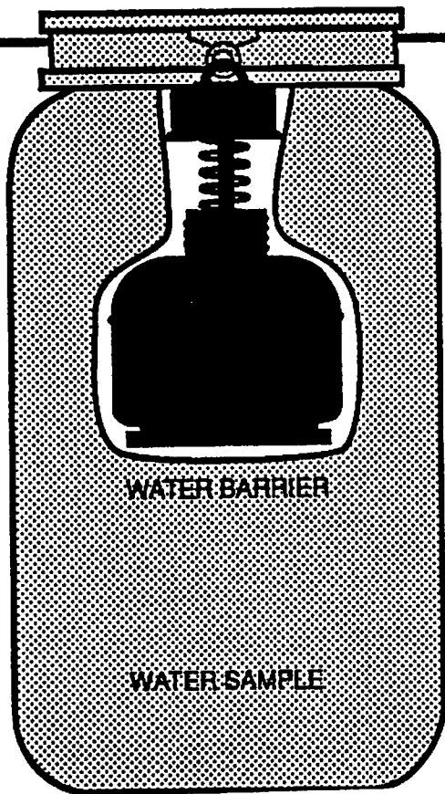
Figure 2 SCHEMATIC OF MEASUREMENT OF RADON AND RADIUM BY IMMERSION METHOD
