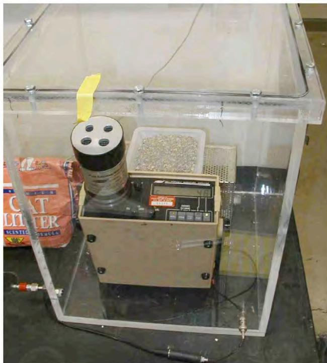
Fig. 1. Photograph of the radon detection system used in the analysis of the cat litters.
