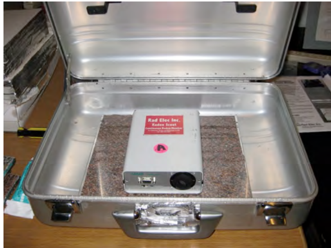
Fig 5 Enclosure accumulator with CRM and granite sample
