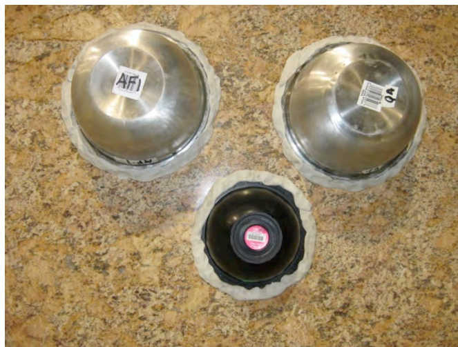
Fig 2 Two discrete component flux monitors and one RFM deployed on a vertical granite surface.
