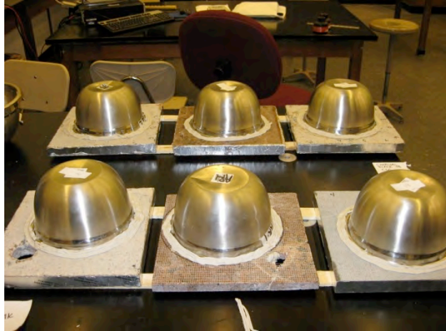
Fig 6 Accumulators applied to the “non-polished” sides of six granite samples
