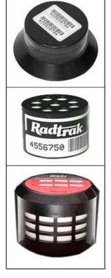
Figure 6. Alpha track detectors. Top-bottom: Accustar, Landauer, RSSI
