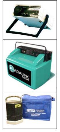
Figure 7. Continuous Radon Monitors
