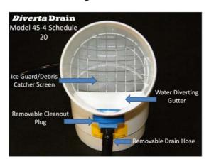
Figure 2 – Features of Diverta Drain
