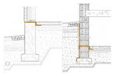
Figure 1. Sealed Bitumen Felt Strip Membrane
