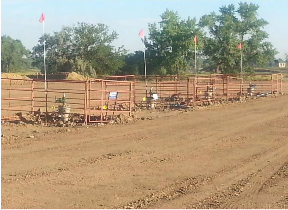
Figure (4): A typical drilling pad with 5 finished wells and sealed well heads. The highest outdoor radon was measured (4.5 pCi/L) at this site.
