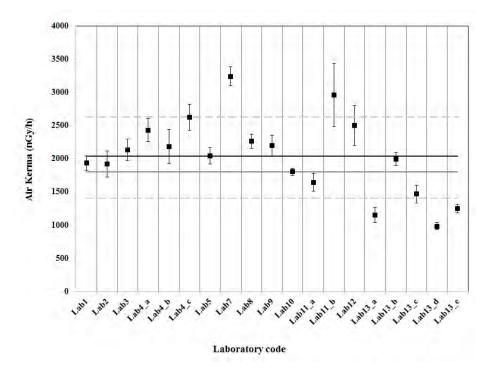
Figure (6): Results of the test in the reference point with high levels of external gamma dose
