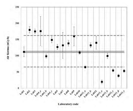
Figure (5) Results of external gamma dose rate in a reference site 110 nGy h<sup>-1</sup>
