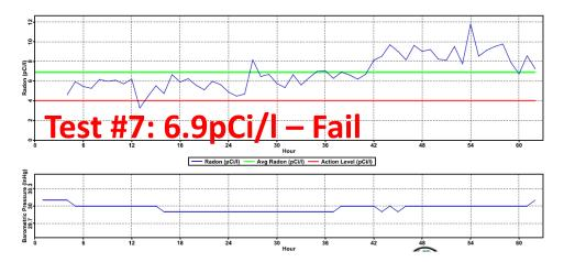
Figure (3): Graphics provided by Radalink for Test #7 showing a failing score of 6.9 pCi/l
