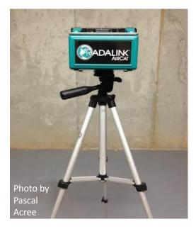
Figure (1): Experimental setup of Radalink AirCat® monitor located in basement of a three story house which had recently tested at the 4.0 pCi/l action level.
