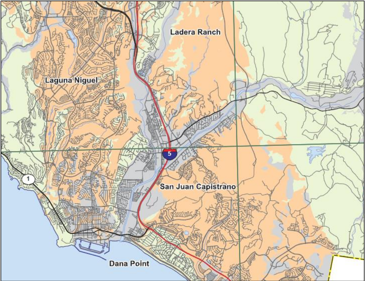
Figure (10): A portion of the Orange County radon potential map showing the typical level of detail for CGS radon maps. Moderate radon potential is orange, low radon potential is green and unknown radon potential is gray (Churchill, 2015).
