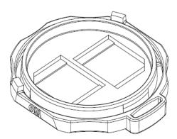
Figure (1): Bottom part of the detector which has two alpha-track film location areas.
