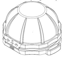
Figure (3): The detector can be turned 180° between the ON and OFF positions. The ON position exposes one CR-39 (e.g., time period of interest) and the OFF position exposes the other CR-39 film (e.g., secondary time period of interest).
