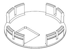
Figure (2): Cover shield with opening in the top of the detector.
