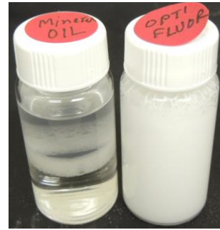
Figure (8b): Sample + Fluid (Opti-Fluor and mineral oil) at 5 hours after mixing.
