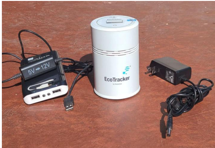
Figure 10: EcoTracker battery setup
