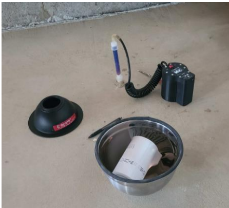
Figure 34: Grab samples and Flux test
