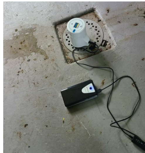
Figure 31: Floor drain measurement
