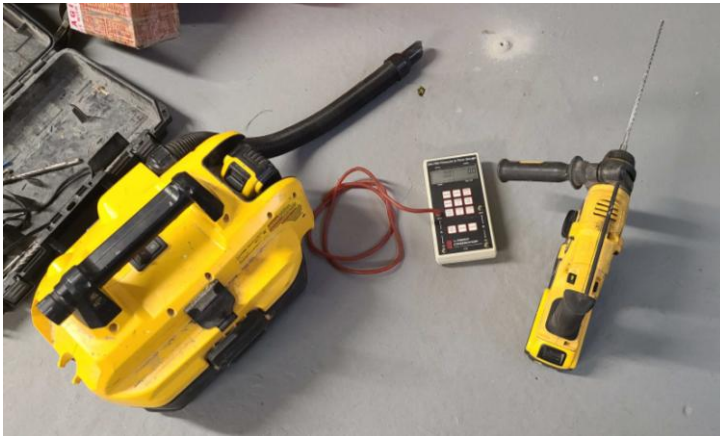
Figure 27: Sub-slab pressure measured 1st
