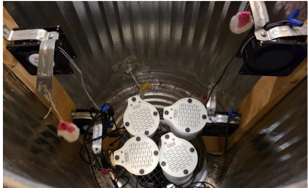
Figure 43: Ecotrackers in Thoron chamber with thoron mantles and circulating fans
