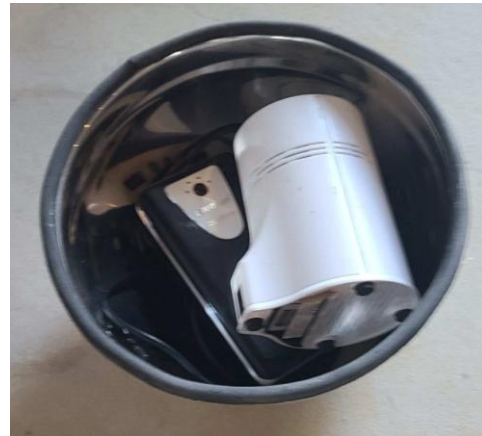
Figure 35: EcoTracker and battery placed in metal bowl
