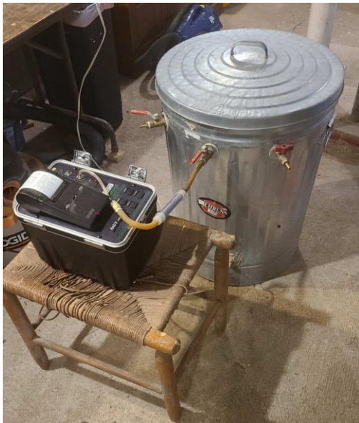
Figure 42: RAD7 measuring Thoron chamber
