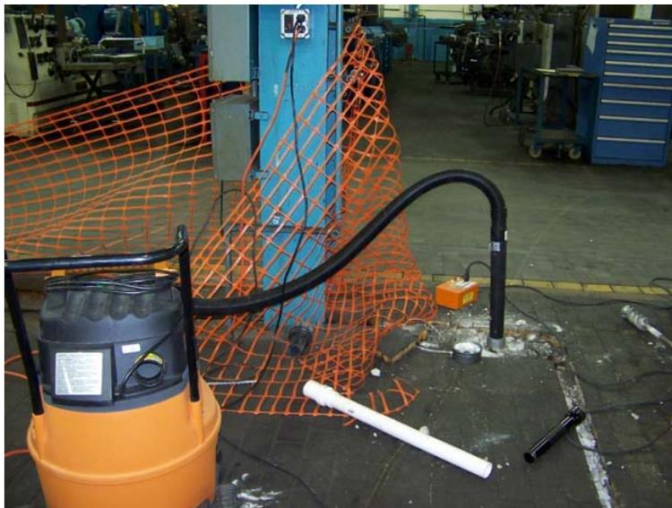
Figure 8 Sub-Slab Communication Test
