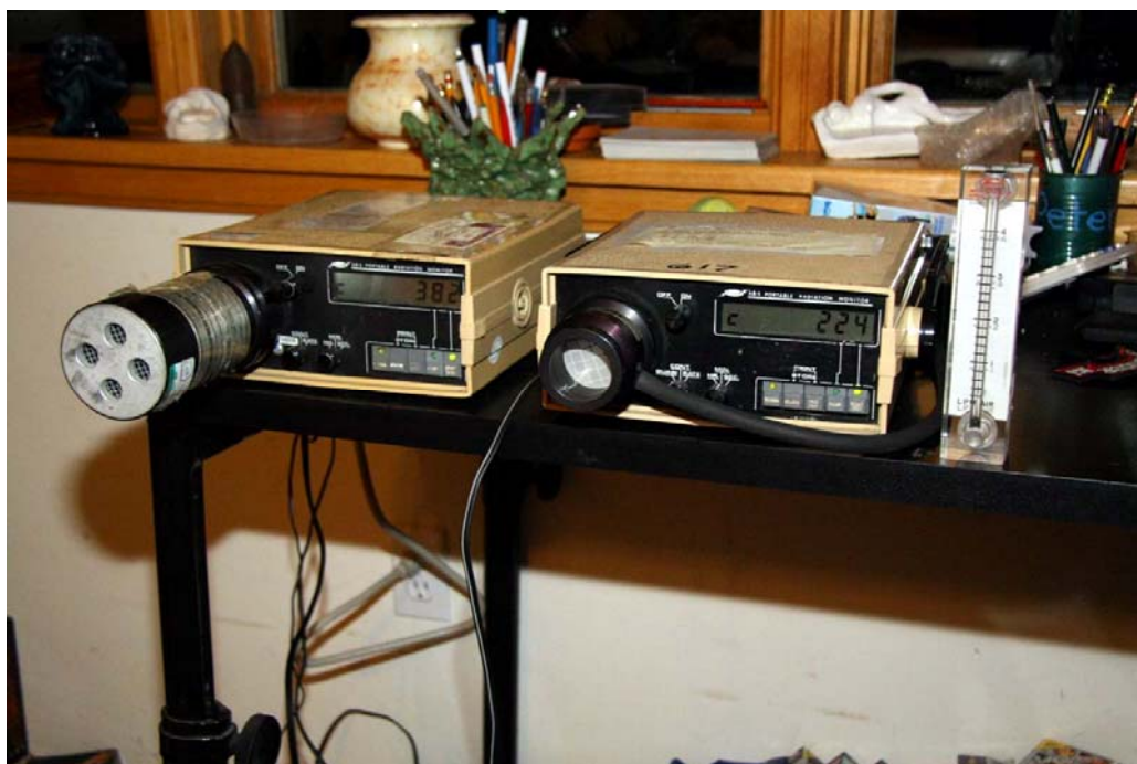
Figure 1 – Pylon AB5 CRM with PRD & Pylon AB5 CWLM with AEP47
