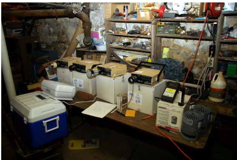
Figure 5 – Portable HEPA filter in front of WL-617
