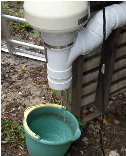
Photo 8 – Drain hole test
