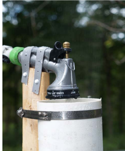
Photo 7 - Nozzle spray into exhaust
