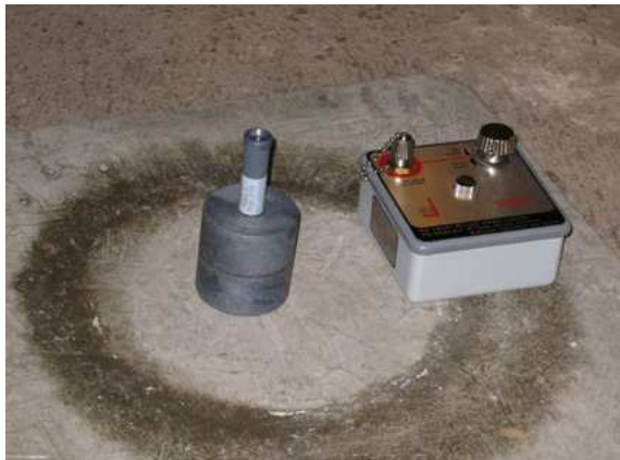
Figure 15 – 2 mR Gamma Dosimeter & re-charger
