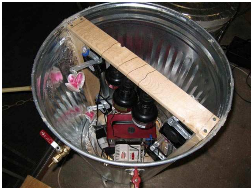
Figure 6 - 114 liter Thoron Chamber using Aladdin mantles & fans
