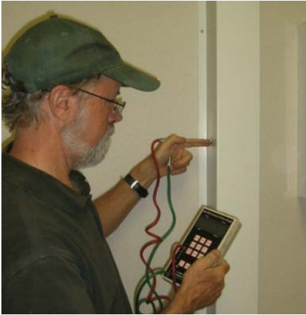
Figure 6: Pitot Airflow Measurement
