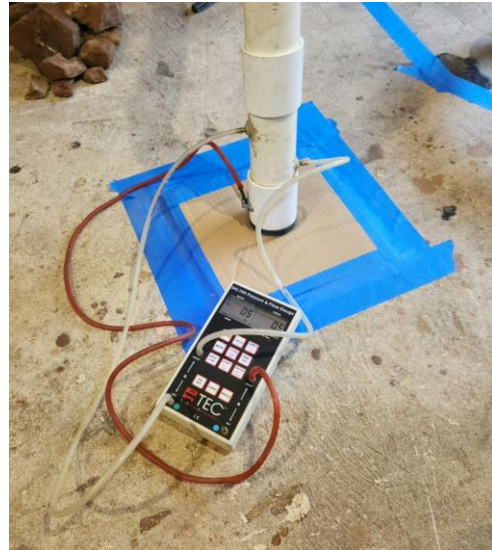
Figure (17): 5-inch core w/full dig out
