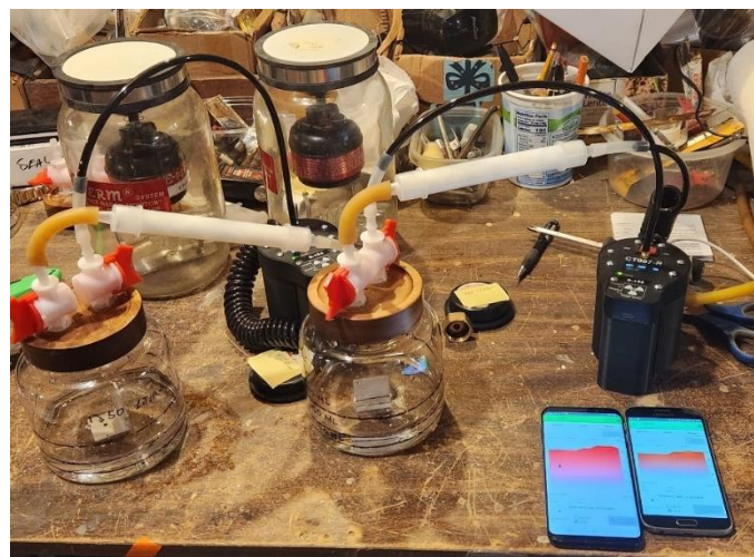
Figure (16): Two water sampling jars being sampled by two RS monitors
