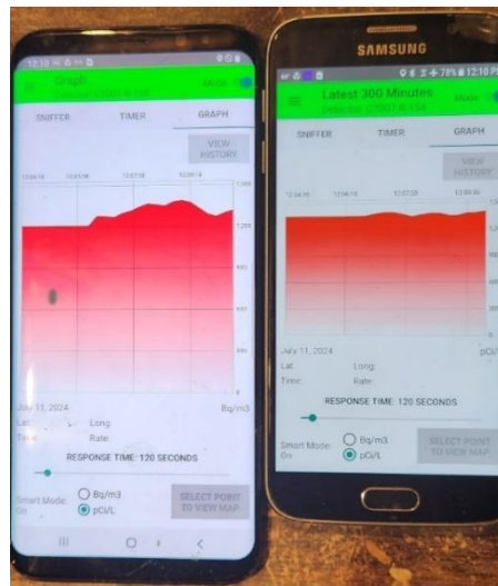
Figure (18) Test 2 - 250mL water sampled 7/11/24 for 10 minutes.
