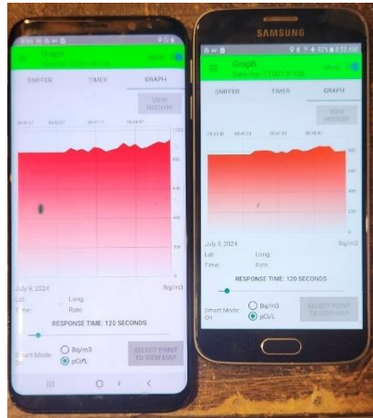
Figure (17): Test 1 - 250mL water sampled 7/9/24 for 10 minutes.
