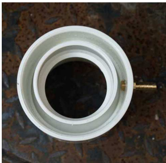
Photo 2 - Top view of 3 to 4 drain
