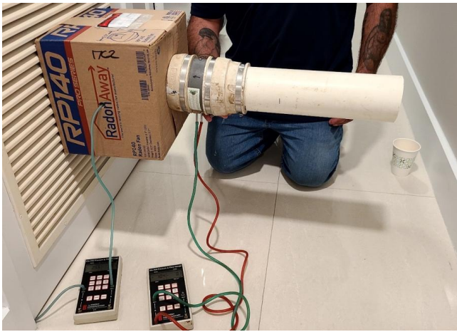
Figure (20): Testing airflow induced by negative AC closet
