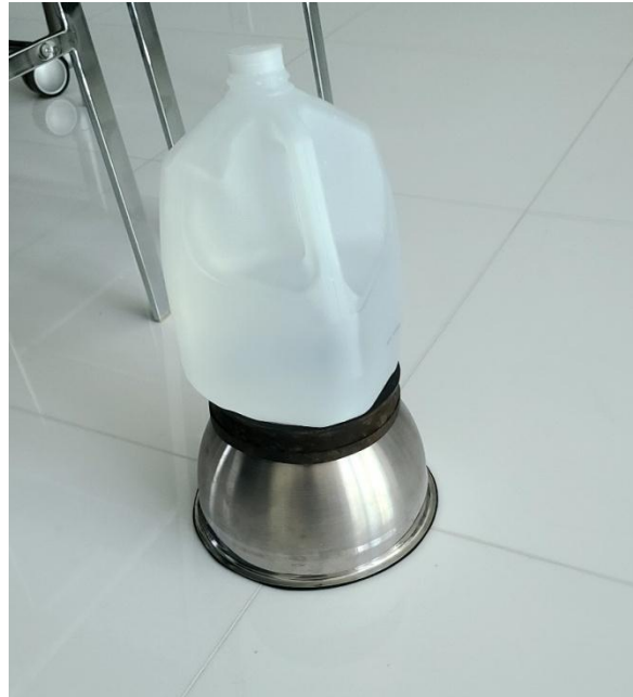
Figure (9): Flux measurement over intersecting grout lines
