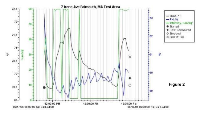
color printer should be used to emphasis the difference in the items graphed when multiple parameters as plotted for ease of reading. This setup had a 30-minute sample rate over a 24-hour period which yielded adequate data and is not too busy. Note that the logging must be stopped by a physical connection to a computer and a software command to stop. Otherwise, it will continue logging until the internal memory is full, collecting additional data that may not be relevant to the placement.
