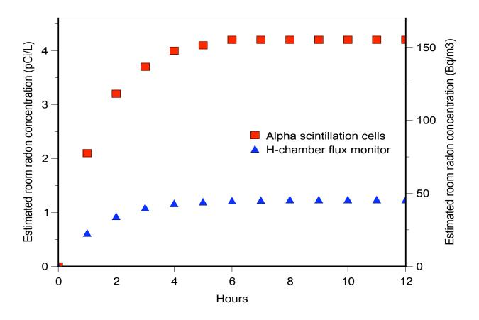
Figure 1. Estimate of radon ingrowth in a 20  $m^3$  room from granite countertop material based on measurements conducted using a H-chamber flux monitor and alpha-scintillation cells.
