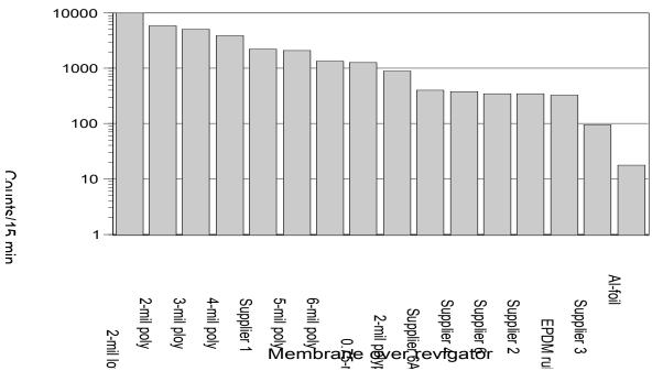
Fig. 4. Count rates measured with membranes separating continuous radon monitor and revigator (repeated setup 2A).
