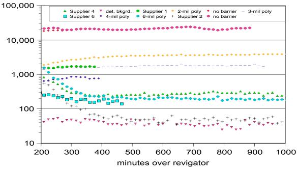
Fig. 3. Count rates measured with membranes separating continuous radon monitor and revigator (initial setup 2A).
