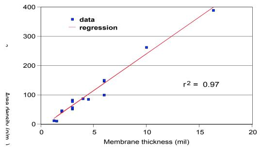
Fig. 1. Membrane thickness is strongly correlated with area density for the materials studied. Table 1. Description of membranes tested.
