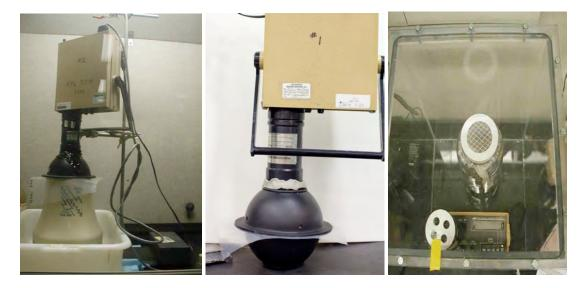
Fig. 2. Experimental setups that were used to examine the permeability of membrane materials: continuous radon monitor mounted over water-filled Revigator (A); <sup>226</sup>Ra capsule and continuous radon monitor (B); and covered glass jar containing <sup>226</sup>Ra capsule in airtight chamber (C).
