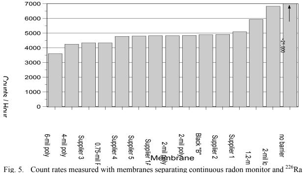
Fig. 5. Count rates measured with membranes separating continuous radon monitor and <sup>220</sup>R capsule (setup 2B).
