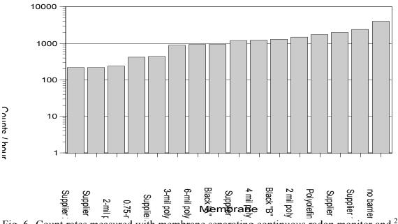
Fig. 6. Count rates measured with membrane separating continuous radon monitor and <sup>226</sup>Ra capsule inside airtight chamber (setup 2C).
