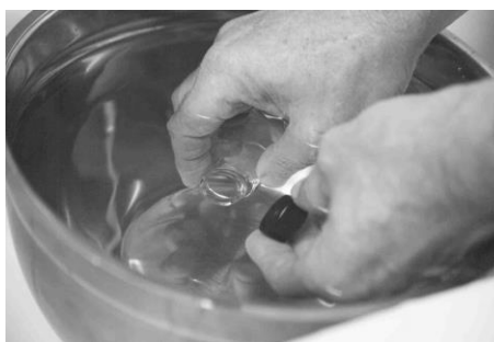
Figure (1): Submerged bottle method of sampling.
