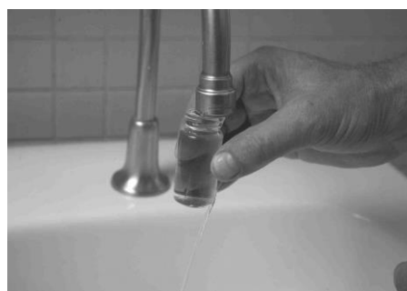
Figure (2): Direct-fill method of sampling.
