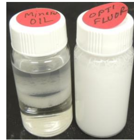
Figure (9b): Sample and Fluid (Opti-Fluor and Mineral Oil) at 5 hours after mixing.
