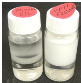
Figure (9c): Sample and Fluid (Opti-Fluor and Mineral Oil) at 68 hours after mixing.
