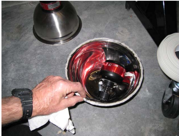
Figure 3 E-PERM placed inside Emanation Bowl with edge sealing
