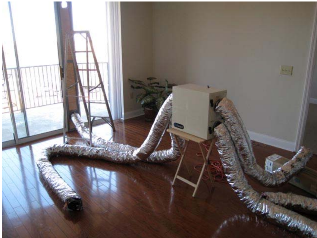
Figure 16 Small ERV being tested for effectiveness
