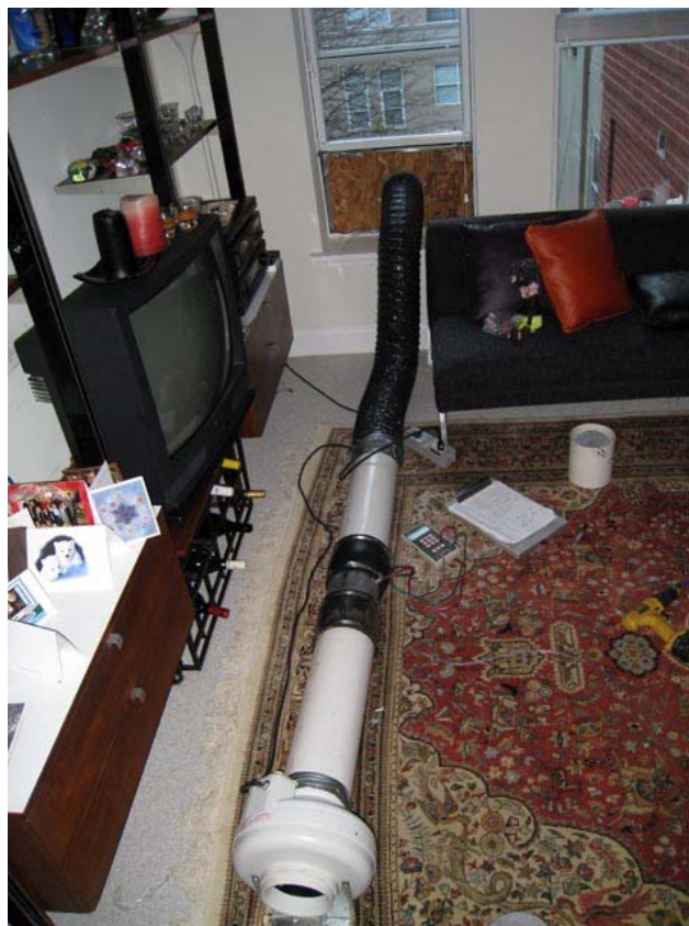
Figure 6 Blower door set up
