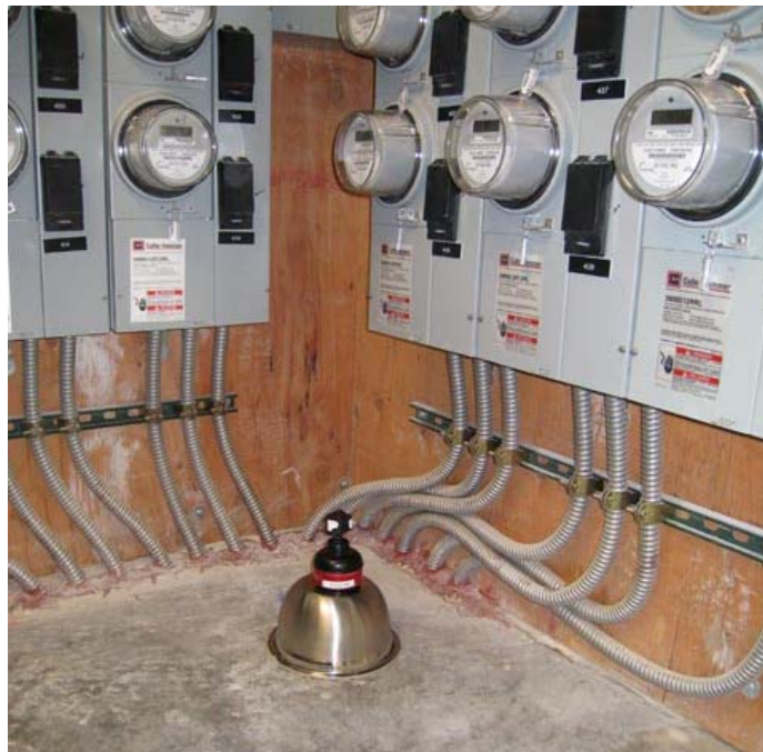
Figure 4 E-PERM Slab Emanation with room air measurement
