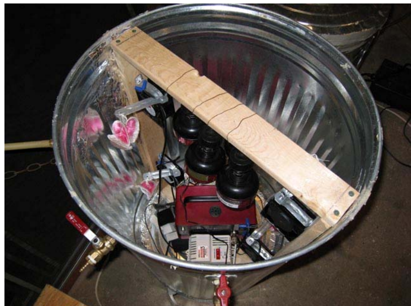
Figure 6 - 114 liter Thoron Chamber using Aladdin mantles & fans
