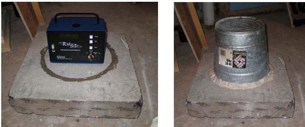
Figure 11 – RS800 sealed under 9.6 Liter Accumulator for Mixed Slab
